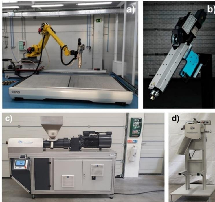
Figure 2: PL15 upgrading a) robotized cell, b) pellets extruder, c) extrusion station and d) pelletizer.
