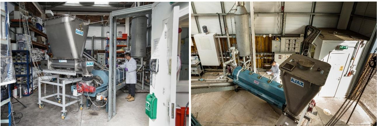
*Figure 10: Upgraded twin-screw feeding system of pilot line 8 (left). Upgraded gas combustion system (right).*
