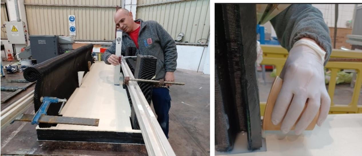
Figure 35: Assembling of all the modules on the left. Railings and columns fixed with epoxy resin on the right.
