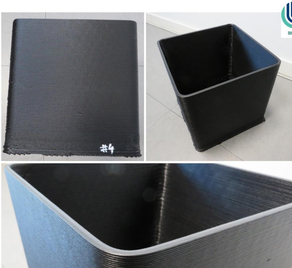
*Figure 17: Printed cubes in PL15 using LIST compounding based in PLA*
