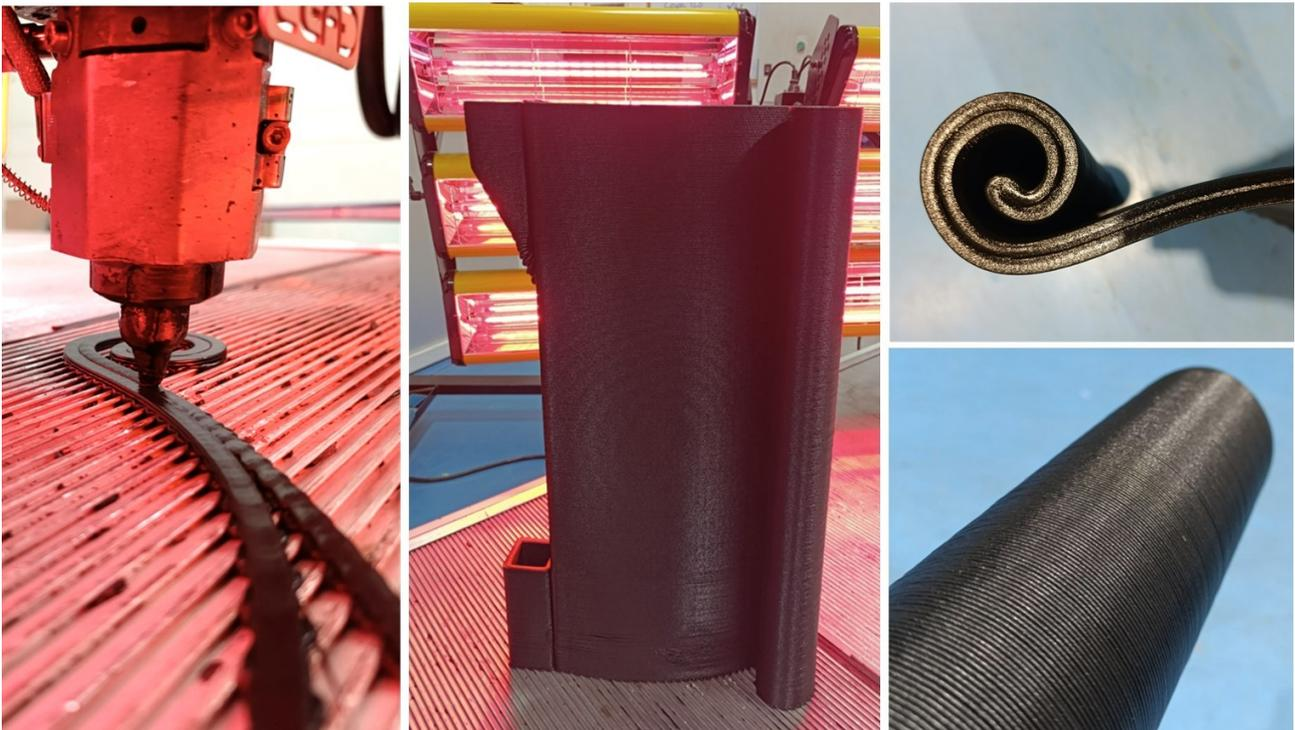
Figure 24: Images of rail type 1 and its printing process.
