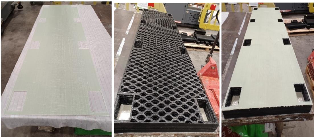
Figure 34: Basement assembling
